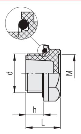
$\begin{array}{lll} d & = M \ 14x1.5 \\ D & = 22 \\ h & = 9 \\ L & = 17 \\ M & = 15 \\ s & = 19 \\ Weight (g) = 4 \end{array}$
